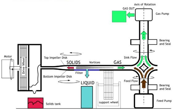
McCutchen Processor for separation of Gases, Solids and Liquids
